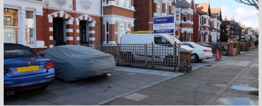
Loss of and paving over front gardens, no planting, and no drainage means water runs onto the street
