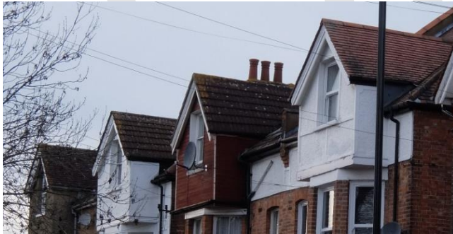
Some of the houses in Buxton Gardens have original loft floors, with overhanging box walls, over a canted bay, with sash windows in the gable end.
